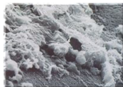
Sand particle with Organic Acid coating causing water repellency
